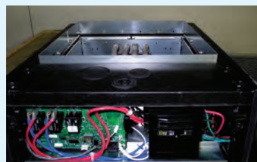
Figure 4 Late model slide-in heater kit using electronically controlled switching relays that are significantly quieter. In the latest designs, the relays remove power from both legs of the heaters when the heating cycle is done.
