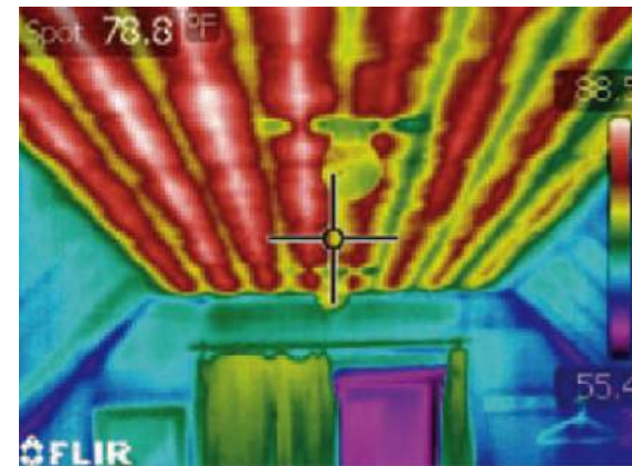
Thermal image of radiant ceiling in operation
